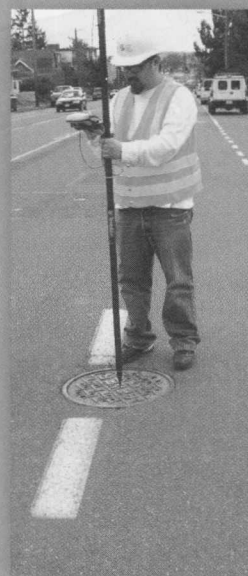
To collect and log location, size, condition, and other data on this manhole, Field Technician Leo Asuan uses a Trimble GeoXH unit, which is equipped with a Zephyr antenna and 6-foot antenna for improved spatial accuracy. Photo: Karen Zollman
